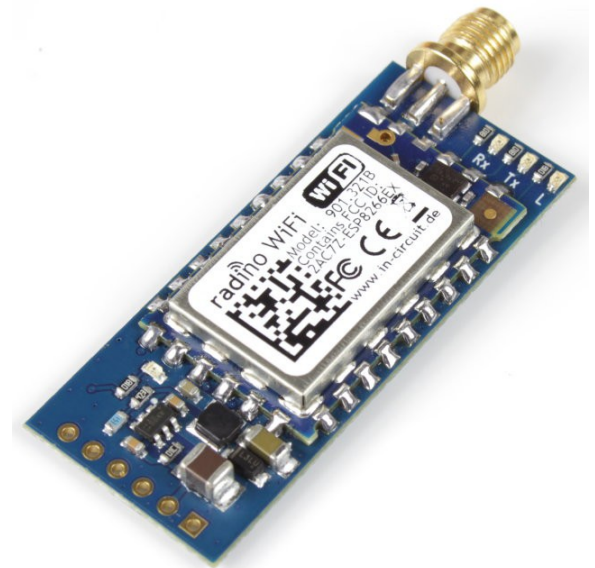
radino UART-Bridge with radino WiFi
