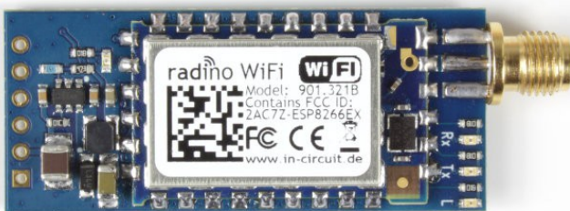
radino UART-Bridge top with radino WiFi
